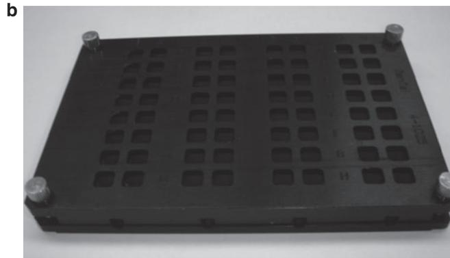
Fig. 3. Parallel processing of 77 samples on eight slides. **(a)** Sample arrangement on eight slides. G1, G2, G3, and G4 are four different groups of samples. Control samples are C1 and C2. B is blank. **(b)** A picture of SIMplex multiwell device.
