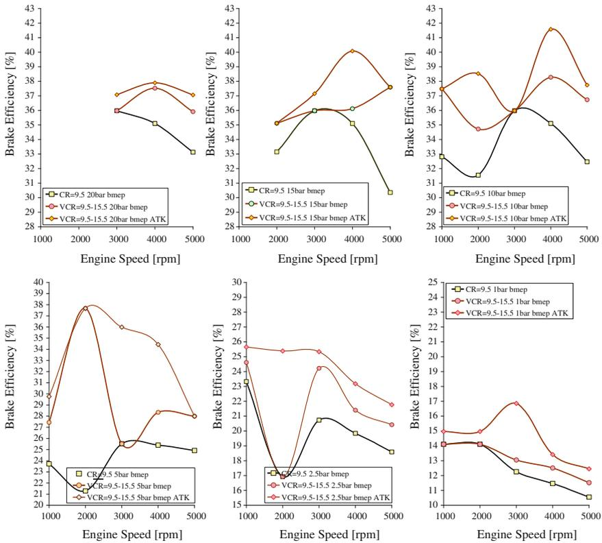
**Fig. 4** Brake thermal engine efficiency with fixed compression ratio, variable compression ratio (maximum efficiency limited by knock) and variable compression ratio and Atkinson effect for operation at various BMEP
