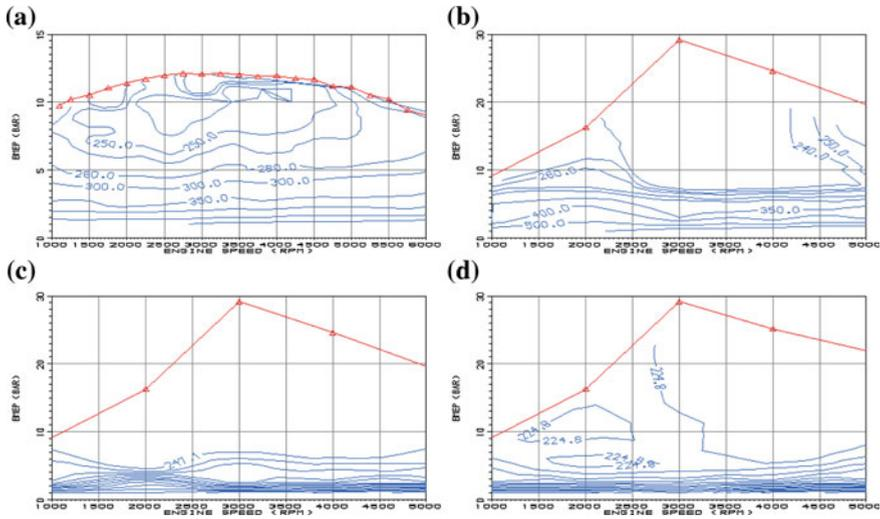
**Fig. 7** Brake specific fuel consumption maps for the **a** 4 L naturally aspirated gasoline engine, **b** 2 L GDI turbo charged engines with fixed compression ratio (FCR), **c** 2 L GDI turbo charged variable compression ratio (VCR), **d** 2 L GDI turbo charged VCR and variable stroke ratio (ATK)
