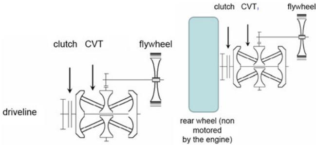
**Fig. 5** Schematic flywheel of the driveline (*left*) and a non driveline (*right*) mechanical hybrid systems
