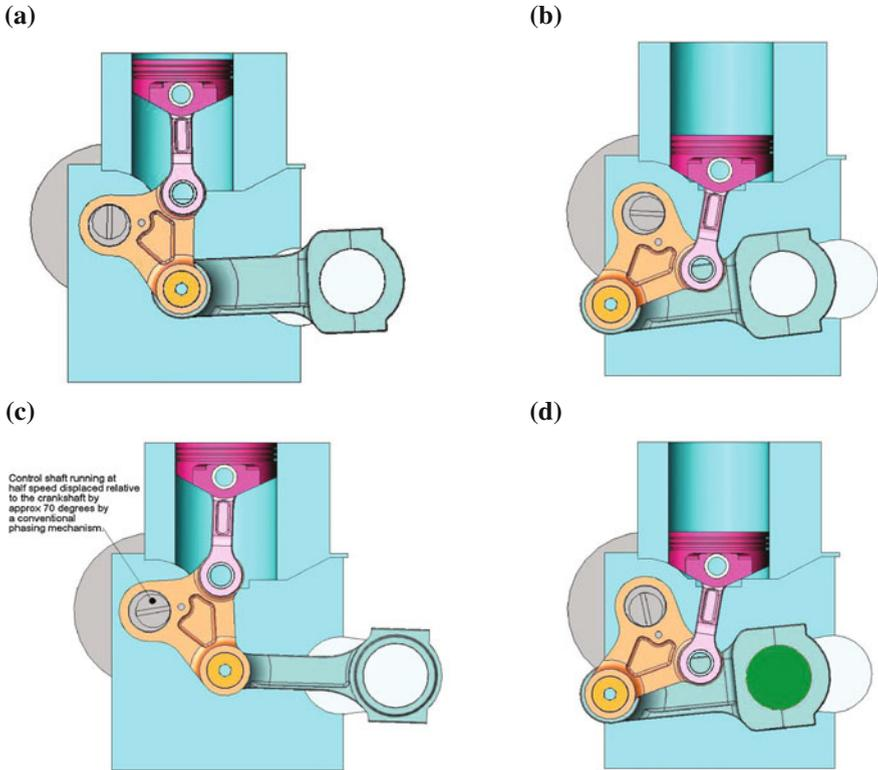
**Fig. 1** Low and high CR mechanism at TDC (a, c) and BDC (b, d)
