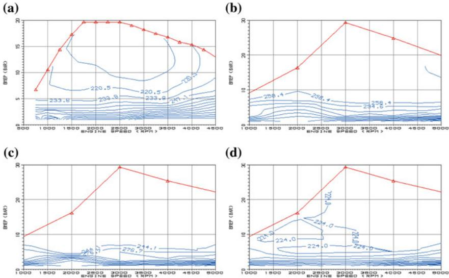
**Fig. 8** Brake specific fuel consumption maps for the **a** 1.6 L TDI Diesel, **b** 1 L GDI turbo charged engines with FCR, **c** 1 L GDI turbo charged engines with VCR and **d** 1 L GDI turbo charged engines with VCR and ATK
